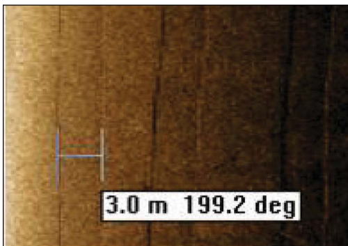
Figure 1. Sidescan sonar sonograms of hydraulic dredging marks (up) and width (down) of furrows left by the dredge on the seabed.
